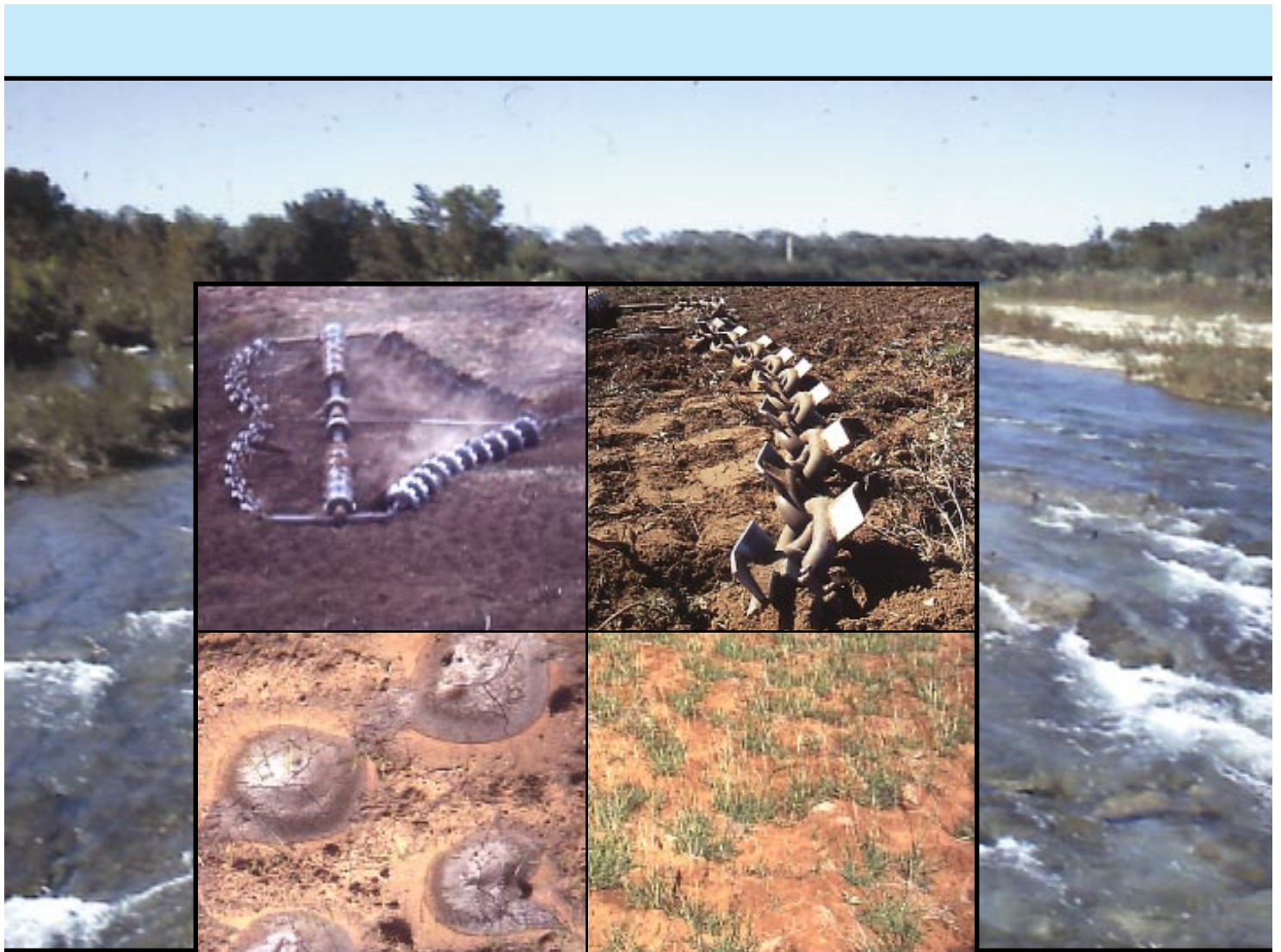
Figure 10. The disk-chain diker designed by Harold Wiedemann, Texas Agricultural Experiment Station, Vernon, Texas, reduces brush and creates pits which concentrate water and nutrients for forage species.
