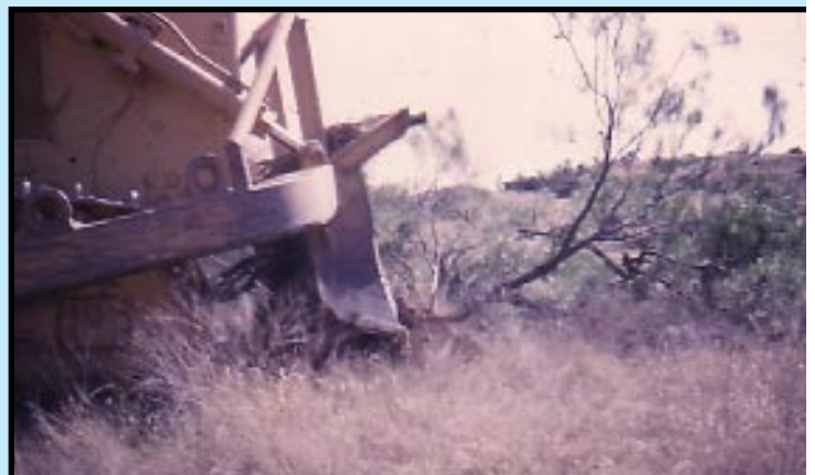
Figure 9. Power grubbing removes water-using brush and creates basins which concentrate water and nutrients for forage plants.
